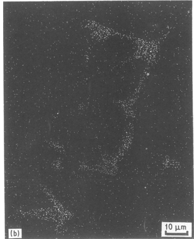
Figure 3 (a) Arrow-shaped carbide morphology. Note that the growth directions (A–B, C–D) of these particles are suggested to be along the \langle 001 \rangle because they are aligned perpendicular to each other. The distribution of major elements is given in (b) and (c), which indicates these particles are rich in Nb and Hf. (b) Nb, (c) Hf.
